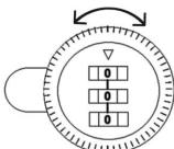
To lock the camlock, rotate the dial back in lock position and scrabble the code
