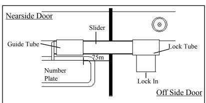
2. With lock engaged in the slider, mark out position of lock tube and guide tube onto rear door with a pencil, unlock slider, then mark out each hole position. (Use a packer plate as a template to mark hole centres).
