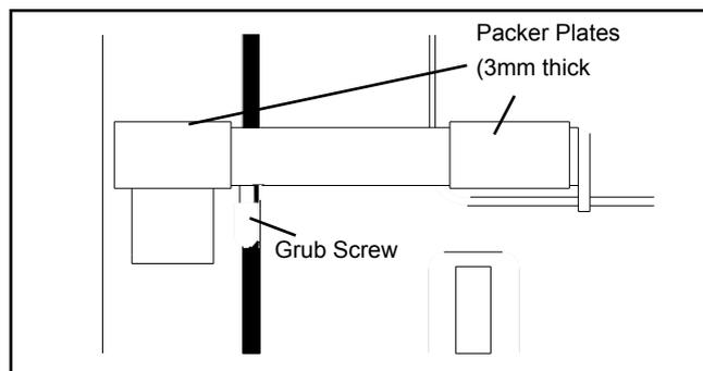
3. Fit the lock and guide tubes to the door pillar and side door with the countersunk fasteners provided using packer plates between the door/door pillar and the tubes as required to gain best alignment. Use 5mm hexagon key to hold the fasteners when tightening.
