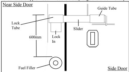
2. With lock engaged in the slider, mark out position of lock tube and guide tube onto door pillar and side door with a pencil, unlock slider, then mark out each hole position. (Use a packer plate as a template to mark hole centres).
