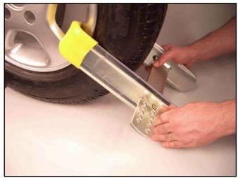
2. Slide inner and outer arms together, ensuring pointed outer arm fits into recess or hole in wheel. Position padlock above the hole closest to the outer arm and turn the key to lock.
