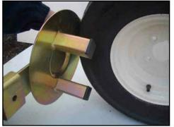
1. With the tyre valve positioned away from the tubes welded to the inside of the Trail Clamp disc, hook the arm behind the wheel.
