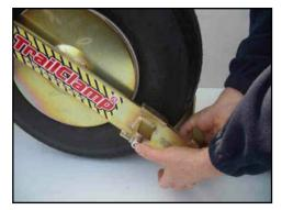
3. With the lock in the unlocked position, slide the return arm in around the rear of the tyre and lock by pressing the plunge lock in until it clicks.
