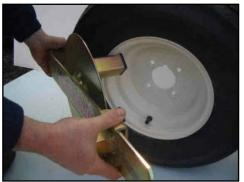
2. With the arm hooked behind the wheel, move the arm of the Trail Clamp in So that it lies flat against the tyre.
