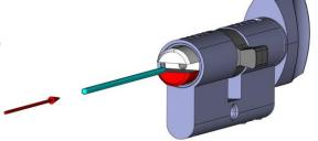
With simultaneous pushing and turning of the colored display, it can be turned by 180°.
