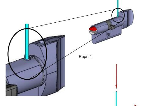
Push slightly and turn the knob at the same time. Remove the pin and bring the cam in assembly position (see repr.2).
