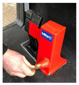
With the key in the lock in the unlocked position insert the lock into the housing.
