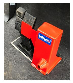
With the lock removed place the cover over the accelerator pedal.
