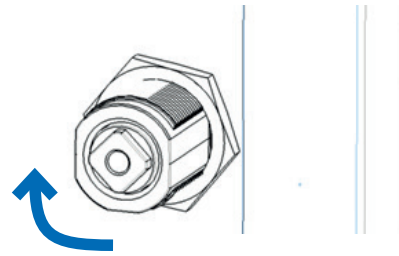
DIAGRAM 2. Fit locking nut & tighten to secure.
