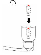
The tumblers are shaped to fit into the slots - The coloured tip **must**be facing upward - The side of the tumbler that has the raised notches must face toward the top of the lock
