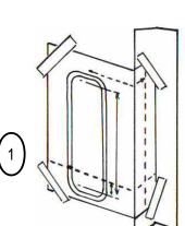
2) Drill the lock holes as per the template to ensure trouble free operation the holes
