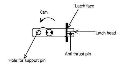
3) Insert the latch bolt into the hole, draw a line around the latch bolt face and remove it 4) Chisel out the lined space until the latch bolt face is flush with the surface of the door edge, fasten latch bolt with wood screws
