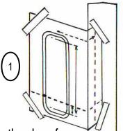
2) Select the strike and mark it's position on the frame before drilling the door for the lock
