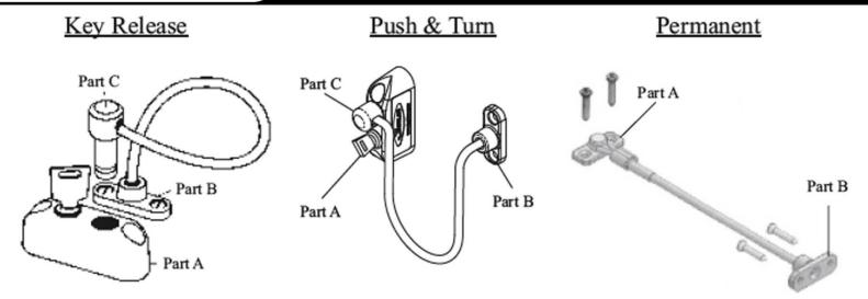
The standard length of the Jackloc cable is 200 mm.
