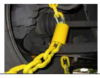
**3.** Collect the chain end from behind the left side of the wheel and pull to take up all the slack in the chain loop.
