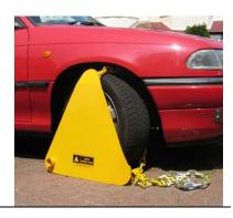
**2.** Pass the unattached chain end around the back of tyre, and over the vehicle's suspension arm
